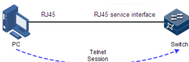
Figure 1-3 Networking with device as Telnet server
